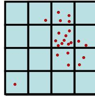
**Figure 8:** Distribution of secondary rays. Each red dot represents a ray in some parametric space (3D origin + 2D direction). Some voxels have none or very few rays, while others have a lot of coherent rays.
