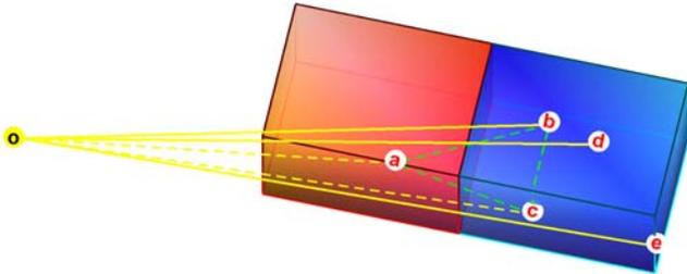
**Figure 2:** Problems using boundary rays as a proxy for the whole group. The ray **oa**, which is inside the convex hull of the 4 corner rays **obcde**, intersects both cells, while all 4 corner rays intersect only the blue cell.
